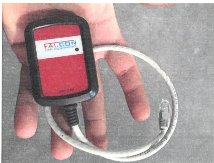
Picture No. 9: Service key that serves to access administration and service menu of the MS2 and PCUx1 electronic calculator
